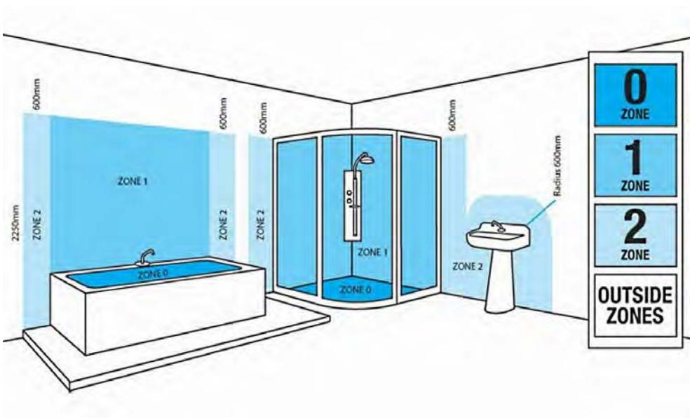
**Zone 0** is inside the bath or shower itself. Any fitting used in this zone must be low voltage, (max 12V) and be rated at least IP67 which is total immersion proof. (We do not currently have any fittings that are suitable for Zone 0).
